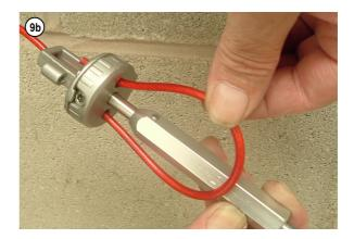
**10a.** The rope is then pulled by hand through the Tensioner / Gripper to take up any slack rope before final locking.
