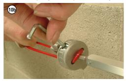
11b. For optimum performance the switch tension should be set at mid position (as indicated by the markers in the viewing window).
