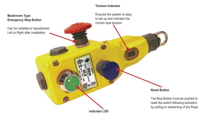
Can be wired to flash RED in the event of the Rope being pulled - switch activated, or illuminate steady GREEN to indicate a reset switch in machine "Run" state. Visible from long distances.
