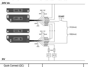
Two switches connected in series to give dual circuit safety outputs to machine contactors.
