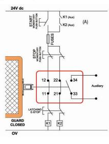
This system shows interlock switch circuits 11-12 and 21-22 configured to allow dual circuit direct feeds to contactor coils K1 and K2. When the start button is pressed and then released, the auxiliary contacts (A) of contactors K1 and K2 maintain the feed to the contactor coils. Opening of the Interlock Switch or depressing the E Stop will isolate power to the contactor coils. Re-start can only occur providing the Guard is closed and the E Stop is reset.
