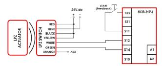
Multiple LPZ / LMZ switches to SCR-31P-i Safety Relay (Viper series):
